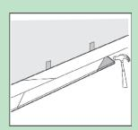
We always recommend an overlap/staggering between end joints to be about 1/3 of the plank length but never less than 300 mm.
