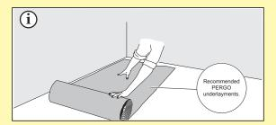
damp screen. Make sure the PE-film overlaps with a minimum of 200 mm. In case of a floating installation with any other type of underlay that is not a Pergo underlay the same technical specifications must be met. In case of problems caused by a non-compatible underlay, no warranty will be valid.
