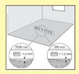
To achieve optimal sound reduction, best walking comfort, avoid squeaking and to level minor unevenness we strongly recommend using a Pergo underlay. A floating installation on cement screed, concrete or in case of floor heating, requires the use of a damp screen. All Pergo underlays have a build-in vapour barrier. In case you use another underlay, which does not have a vapour barrier, the installation of a 0,2 mm PE\_film is required as a minimum
