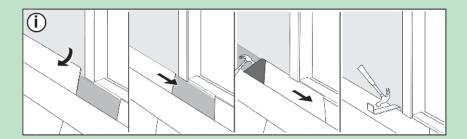
To install Pergo wood flooring around pipes, carefully measure and mark the planks with the exact centre point for each pipe. Drill a hole at each of the marked points that is equivalent to the diameter of the pipe + 16 mm in dry climate and 24 mm in wet climate. If located on the long side of the plank make a 45 degree cut from each hole to the edge of the plank and then cut between the holes as shown. If located on the end of a plank
