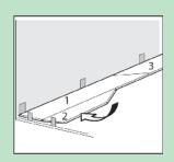
Take plank 3 and 4 and tap them separately into the previous plank, For plank 3 this will be plank 1 and for plank 4 this will be plank 2. If the joint remains slightly open tap it in with a rubber hammer and tapping block.
