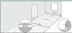
Before starting carefully measure the length and the width of the room to plan a precise lay-out to achieve a balanced appearance of the floor. This will ensure also you won't end up with the last row being too narrow. If the last row would be less than 100 mm the installation will be easier if you cut down the planks of the first row in the length.
