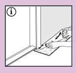
To install Pergo wood flooring around pipes, carefully measure and mark the planks with the exact centre point for each pipe. Drill a hole at each of the marked points that is equivalent to the diameter of the pipe + 16 mm in dry climate and 24 mm in wet climate. If located on the long side of the plank make a 45 degree cut from each hole to the edge of the plank and then cut between the holes as shown. If located
